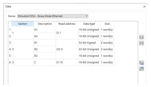
Example 2: Tag-based PLC. The following setting aims to read multiple address tags at a time.
