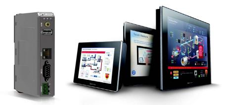
Weintek's newer cMT line of HMIs offer two suites of functions with diverging (and uniquely applicable) capabilities. Newer X-series HMIs have capacitive touchscreens for intuitive gesture control. In contrast, screenless HMIs such as the cMT-SVR-200 shown here uses wifi to connect with local and offsite display devices.
