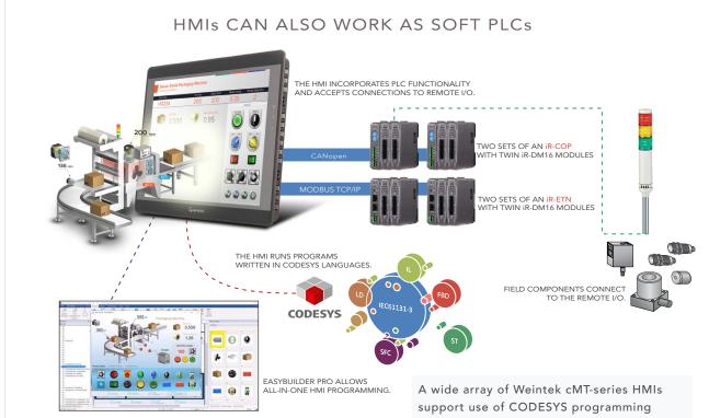
running projects can visualize on the HMI with configuration done through Weintek's programming environment, which is called EasyBuilder Pro (EBPro). Despite some changes in the automation industry over the last few years, CODESYS remains most common for its supports of five programming languages. In fact, CODESYS excels for PLC setup.
