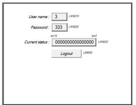
Click [Logout] button to log out, the system will return to the initial state, and current user can only operate class "None" objects.
