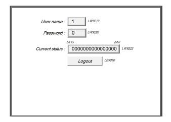
Before entering the password, it displays "0000000000000000000, which means that the user operable object class is "None". [Class A Button] ~ [Class C Button] objects are classified from "A" to "C" and selected [Made invisible while protected]; therefore they are hidden at this moment.
