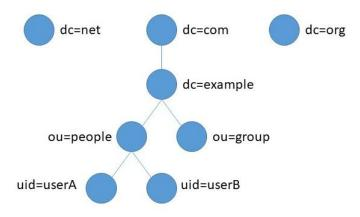
The control addresses used by LDAP Mode are the same as the control addresses used by Enhanced Security Mode. Please see chapter 10.3 in this user manual for more information on the control address. Please note that obtaining LDAP user name using Option List object is not possible; therefore, [Log in by user index] is not supported.
