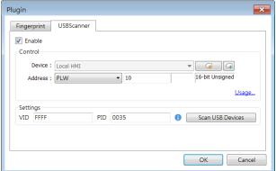
When configuring the USB scanner, to prevent interference from other USB devices during login, it's necessary to first set the VID and PID of the USB scanner. After clicking [Scan USB Devices], the system will prompt a message "Please insert your USB Device". Once the USB scanner is inserted into the PC, the system will obtain a unique VID and PID for the USB scanner. Click [Save], and the system will automatically incorporate this VID and PID into the settings.
