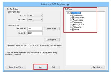
7. To connect another BACnet/MSTP unit, please add the **BACnet/MSTP** driver in EasyBuilder System Parameter Settings again. The communication parameters will follow the settings of the firstly added unit. The way to get tag information is the same
