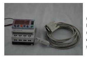
(3m serial link cable) Note: Please use 3m serial link cable (Accessories from Millenium 3) and extension cable (as shown) to communicate with HMI series.
