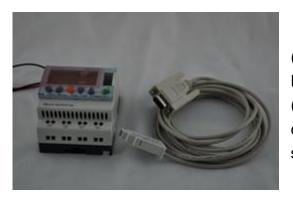
(3m serial link cable) Note: Please use 3m serial link cable (Accessories from Millenium 3) and extension cable (as shown) to communicate with HMI series.
