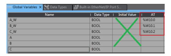
4. %H and %W are 16-bit addresses, so the following mapping method is recommended for better communication efficiency.
