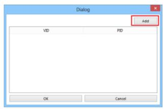
2. Connect the USB Device to the PC and it will automatically detect and pop up a dialogue window.
