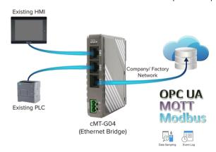
cMT-G04 can be configured by the following ways. Way1. Connect cMT-G04's LAN port with a PC, and on the PC open a web browser and then enter: <a href="http://169.254.0.1">http://169.254.0.1</a>, password: 111111.
