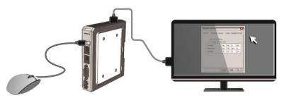
When the cMT-FHDX powers up and the TV displays an image, click the round Start Button in the upper-left corner to open the Setting page. To configure the network, go to the Network tab, click "configure", and a login window will appear. The settings can be modified by entering the system password (default: 111111). In the Setting page, you can see device information, configure general settings, set HMI Time/Date/Name, and more.
