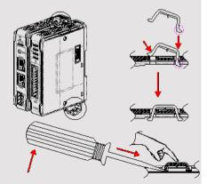
Rail mounting: DIN rail 35mm.
