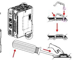
Rail mounting: DIN rail 35mm.
