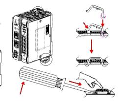
Rail mounting: DIN rail 35mm.
