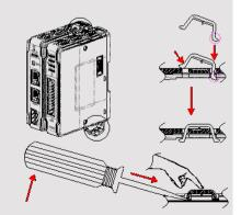
then lift up the screwdriver. Placing a finger on the clip when lifting the screwdriver can prevent the clip from jumping away. The clip can also be removed directly by hand.
