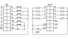
DI: 24x24VDC (Sourcing or Sinking)
