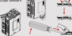
screwdriver into the gap on the clip and then lift up the screwdriver. Placing a finger on the clip when lifting the screwdriver can prevent the clip from jumping away. The clip can also be removed directly by hand.
