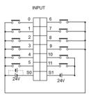
DI: 24x24VDC (Sourcing or Sinking)
